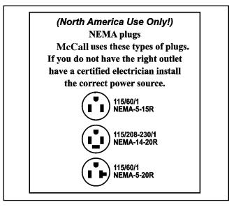
Figure 3. Plug Configurations
