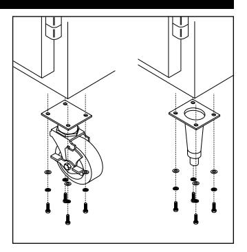
Figure 1. Leg or Caster Installation
