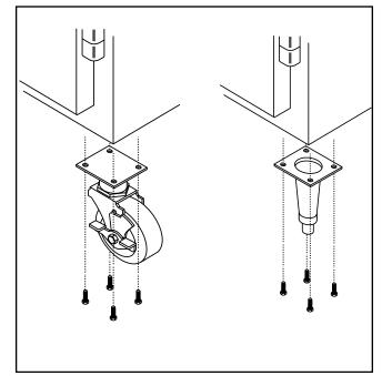
Figure 1. Leg or Caster Installation
